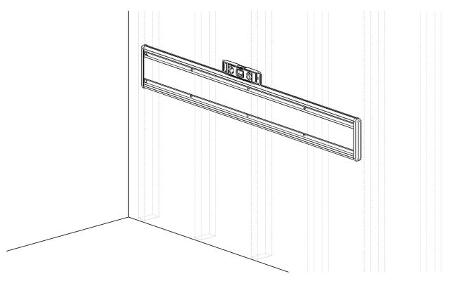
Press-fit the End Caps on both ends of the Handi Tool Rail. Drive a screw through both slots and into each stud in the wall for the maximum weight capacity. Color Strips can be inserted into each slot to completely hide the screw heads.
